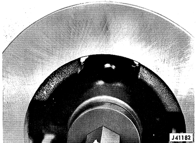
Fig. 2G-58 Correct Rotor Finish (Nondirectional Crosshatch Pattern)
