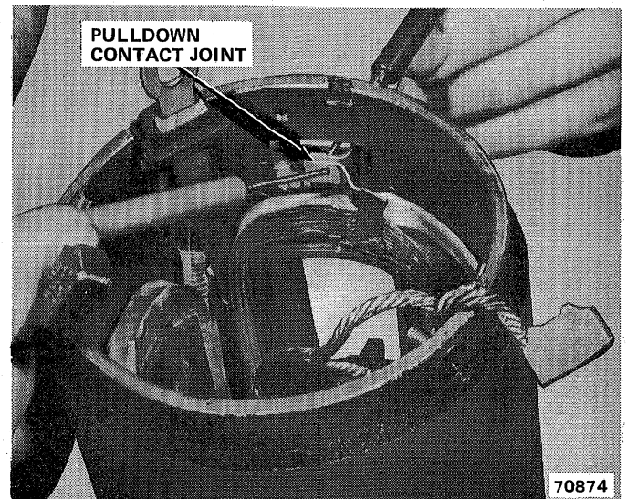
Fig. 1F-17 Solenoid Contact Points Connection Test
